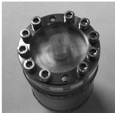
Fig. 4 Assembled swirl element: a) profile view, and b) end view of acrylic section.
